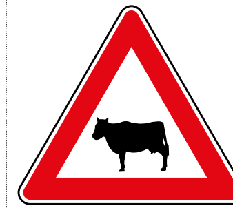
Passage d'animaux domestiques انتبه حيوانات Cattle likely to be in road ahead
